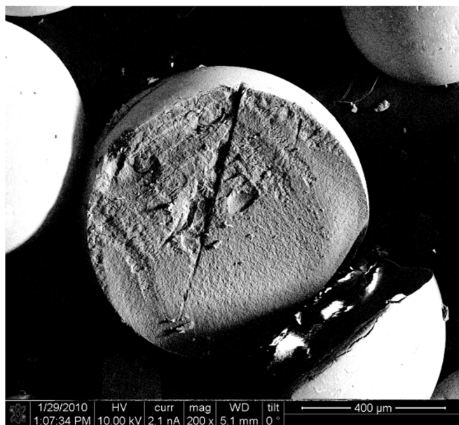
Figure 2a. Focus Ion Beam/Scanning Electron microscope image of a crosssection of titanium dioxide-based hybrid ion-exchange media. Even distribution of white areas throughout the media implies even distribution of heavier elements such as titanium.
