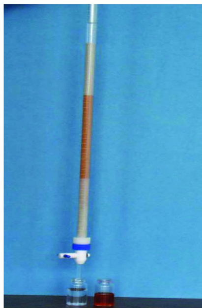
Figure 4. A SPIM “sand-wich”. Treated polycation-micelle sand is layered between untreated sand and Orange OT (in MeOH-water) is eluted. All dye is trapped in the SPIM layer.
